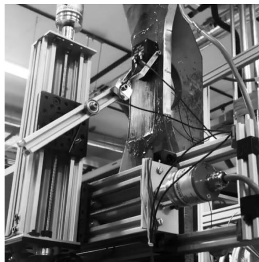
Manipulator developed for test specimen type 1, "rat hole" specimen
