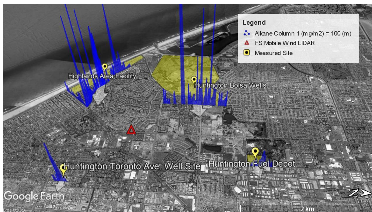
Figure 19. SOF alkane columns (blue overlay) from Huntington Beach sources (survey D), Oct 31, 2019. The figure is a composite of different measurement transects taken between 1:30 pm and 3:30 pm. The wind directions are indicated by the white arrows. Map from Google Earth™, 2020.
