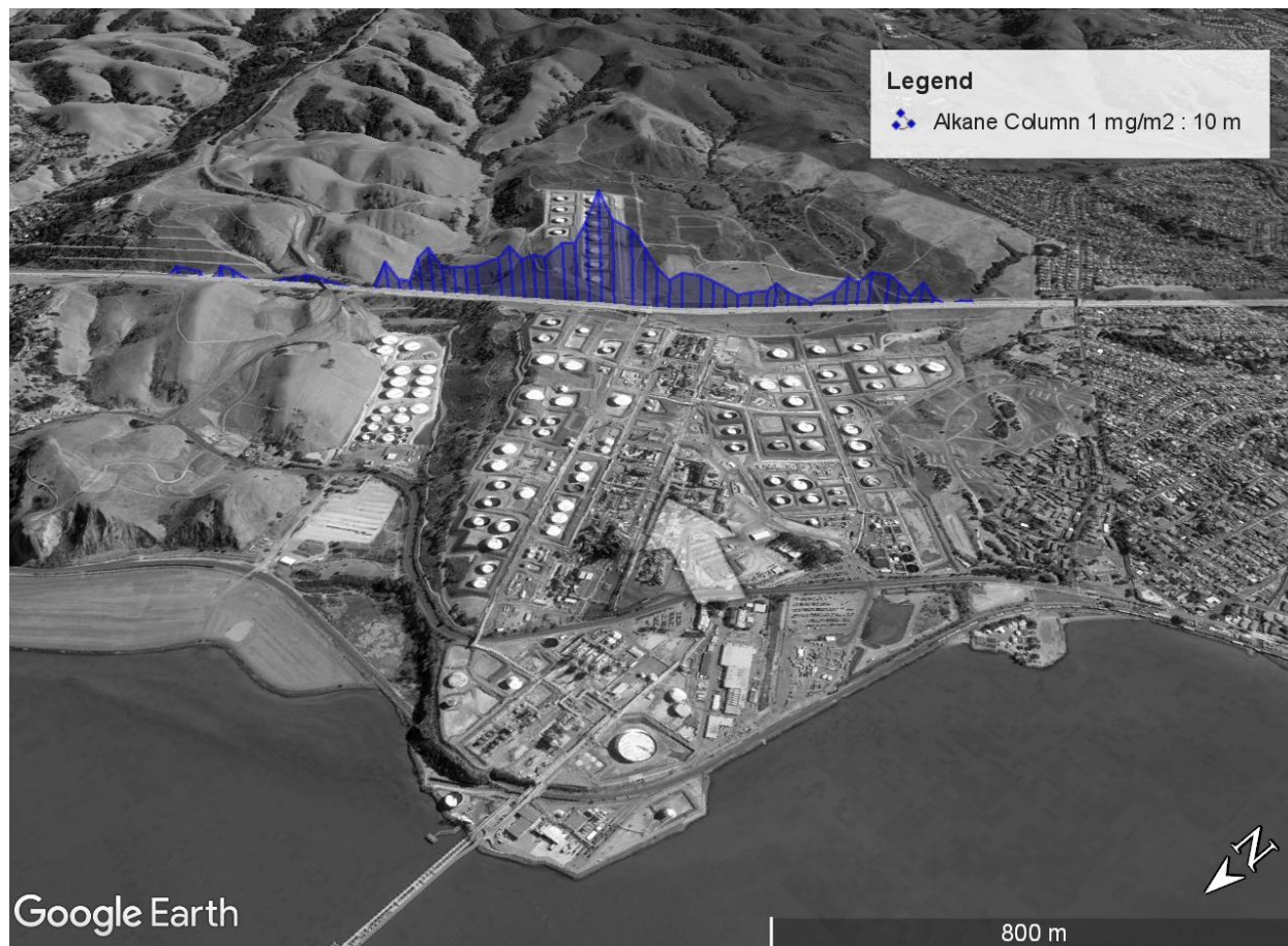
Figure 9. Example of a SOF measurement of alkane emissions at the Rodeo refinery area, survey A, Oct 12, 2018, 2 PM. The apparent height of the blue overlay is proportional to the alkane column. Wind direction during the measurement shown with a white arrow. Map from Google Earth™ 2021.
