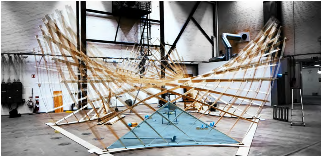
Figure 9: The mechanism in the system was apparent and triggered by motions in the tangent plane. While in motion the rigid parts system could be read, three triangles along the boundaries of the baseplates, coloured blue in this picture. More investigations could be done to find strategies the most optimal places to lock the system using a minimum amount of bracing.
