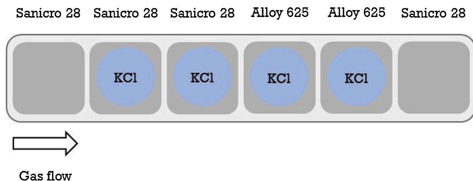
Fig. 1. A schematic drawing of the exposure setup, showing the two sample pieces without and the four sample pieces with the KCl pellets.
