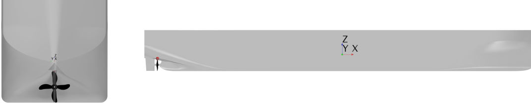
Figure 1: LDP vessel geometry, point probe and ship-fixed coordinate system at COG.
