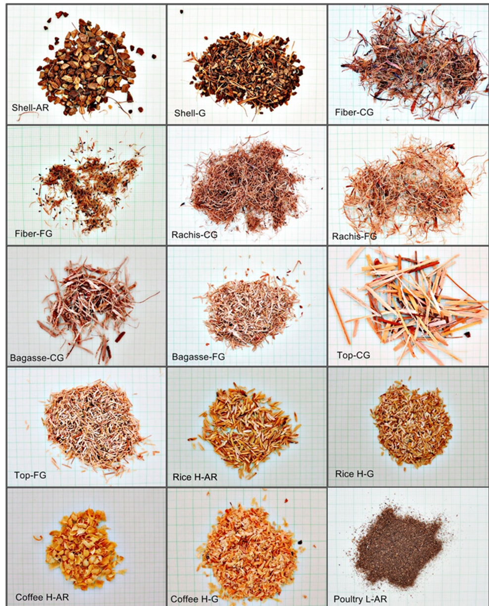
Fig. 1 Pictures of the biomass samples after the conditioning processes: oil palm shell as received (Shell-AR), oil palm shell ground (Shell-G), oil palm fiber coarsely ground (Fiber-CG), oil palm fiber finely ground (Fiber-FG), oil palm rachis coarsely ground (Rachis-CG), oil palm rachis finely ground (Rachis-FG), sugarcane bagasse coarsely ground (Bagasse-CG), sugarcane bagasse finely ground (Bagasse-FG), sugarcane top coarsely ground (Top-CG), sugarcane top finely ground (Top-FG), rice husk as received (Rice H-AR), rice husk ground (Rice H-G), coffee husk as received (Coffee H-AR), coffee husk ground (Coffee H-G), and poultry litter as received (Poultry L-AR)
