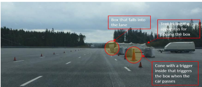
Figure 2: Photograph of test scenario with a suddenly tipped-over obstacle on a two-lane road.
