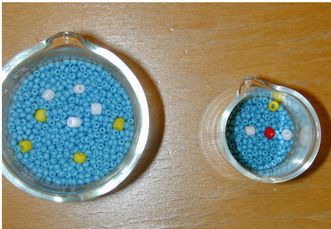
Figure 3. Initial “solutions” are prepared for direct IDA. Left, unknown solution; right, reference solution. Color key: yellow = analyte “A”, red = radioactive “A”, white = reagent “B”.
