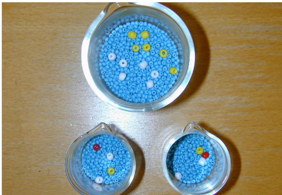
Figure 5. Initial “solutions” for substoichiometric IDA. Top, unknown solution; bottom, the two identical reference solutions. Color key: yellow = analyte “A”, red = radioactive “A”, white = reagent “B”.
