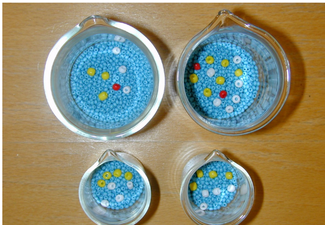
Figure 7. Preparation of the model for IDA-assisted NAA. Clockwise from top left: the unknown sample, the standard sample, and the two identical carrier (reference) solutions. Color key: yellow = analyte “A”, red = radioactive “A”, white = reagent “B”.
