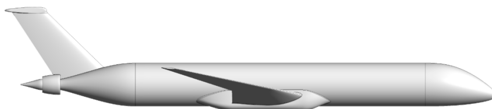
Figure 8. Side-view of the aerodynamic model of the PFC, including wing and vertical tail.
