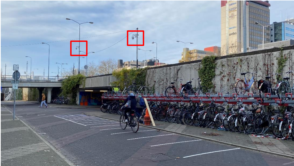
Figure 11.3: Implemented nudge along the through traveling cycling facility, showing two of the three implemented cameras (red boxes)
