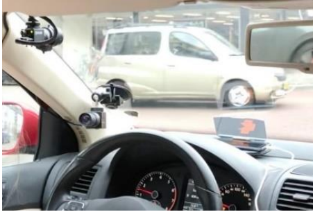
Figure 6.2: The HMI integrated as a HUD in between the steering wheel and the windshield.
