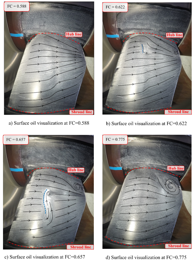
FIGURE 5: Oil-film visualizations on a thick OGV suction side at on-design flow coefficient (0.622) and three off-design flow coefficients (0.588, 0.657, 0.775)
