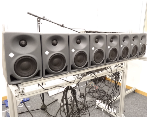
Figure 1 – Example prototype using 8 Neumann KH 80 DSP loudspeakers with a spacing of 154 mm
