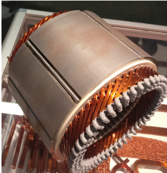
Figure 2.2: Hairpin winding with welded and potted end connections on one side.
