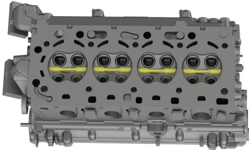
Figure 1. Illustration of sample extraction from the valve bridge regions of the cylinder heads for fatigue testing.
