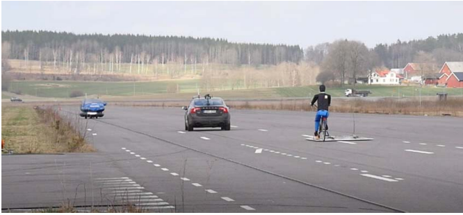
Fig. 1. Test track scenario with ego vehicle (black), robot cyclist, and robot oncoming vehicle (blue). For a video, see https://youtu.be/AixQ189hMi4 .
