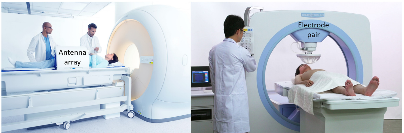
Fig. 1. Example of two RF hyperthermia systems: radiative-based BSD-2000 3D/MR courtesy of Pyrexar Medical, USA (left); and capacitive-based Thermotron RF-8EX courtesy of Yamamoto Vinita, Japan.
