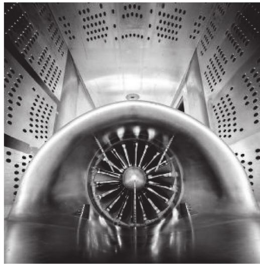
Figure 3. High-speed testing of the distortion tolerant fan propulsor at the NASA Glenn Research Center 8' × 6' wind tunnel [86].
