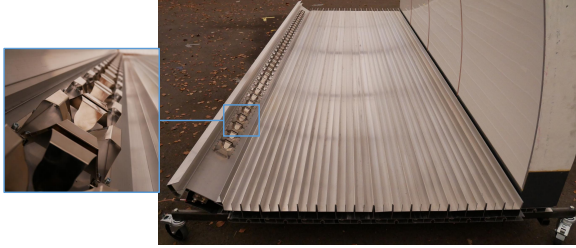
Fig. 2. The feed array of 32 dual-polarized bowtie antennas, plus two extra elements on each side, mounted on the base of metal corrugations in front of the cylindrical reflector antenna.
