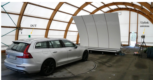
Fig. 19. Picture of the 2 \times 2 MIMO measurement setup for the Volvo V60. A MIMO reference antenna is mounted in the position where a shark-fin antenna normally is located.
