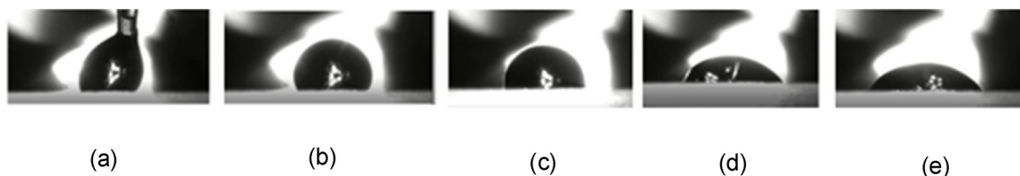
Fig. 2. Wetting process after treatment. When a drop of deionized water is placed over the treated sample the final contact angle does not set instantly: (a) t = 0 s (b) t = 2 s (c) t = 11 s (d) t = 44 s (e) t = 1.36 min.
