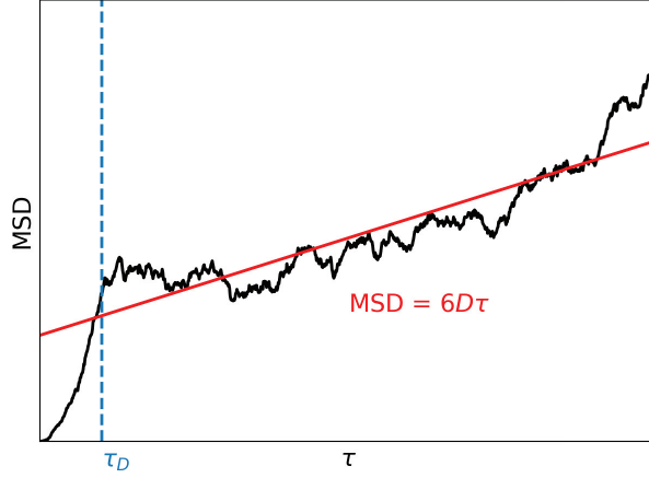
Figure 2.4: Schematic MSD curve, showing also \tau_D , the diffusion onset time and the linear fit used to compute D .
