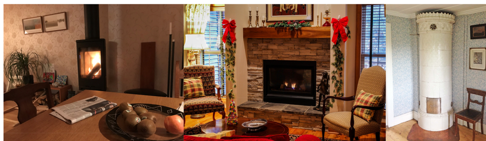
Fig. 2. Different kinds of wood burning appliances. From left to right: a modern wood stove with visible fire, an “open” fireplace, and a ceramic/tiled stove/masonry heater (image credit: Kakelugn med jugendkrön från Rörstrand, ca 1900, by Svante Tirén, CC BY-SA 3.0 license).
