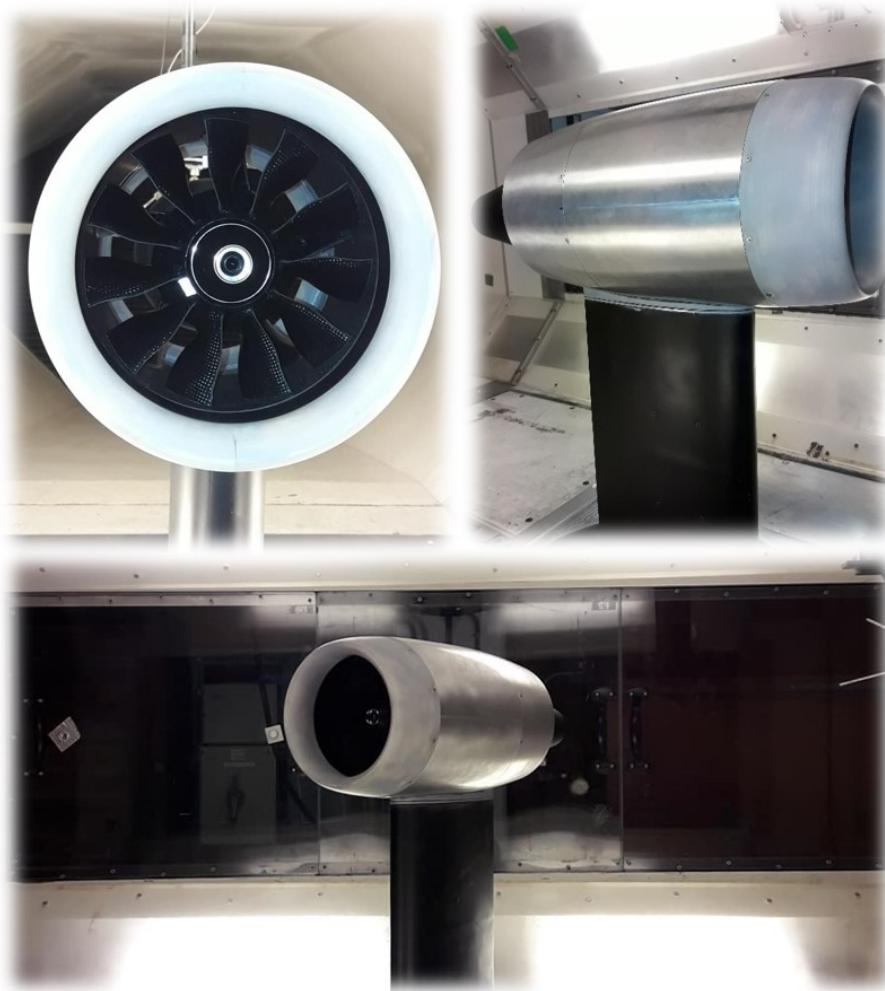
Figure 4.2: Nacelle rig mounted in the wind tunnel.
