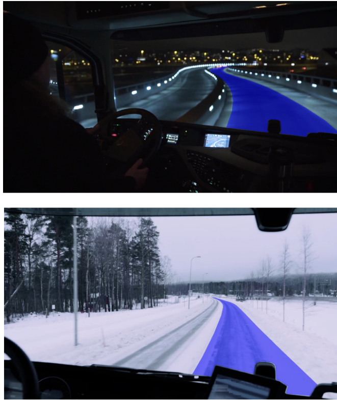
Figure 4.1: Illustration of the road path available via vehicle localization and the road coordinates in different driving conditions (courtesy of Volvo Trucks, altered from the Volvo original images according to the approval).
