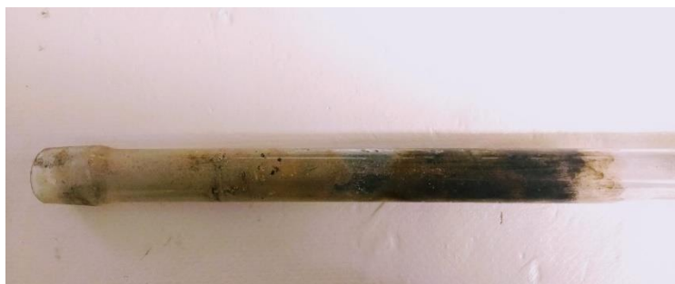
Figure 29: The internal section of the quartz tube covered with the organic by-product.
