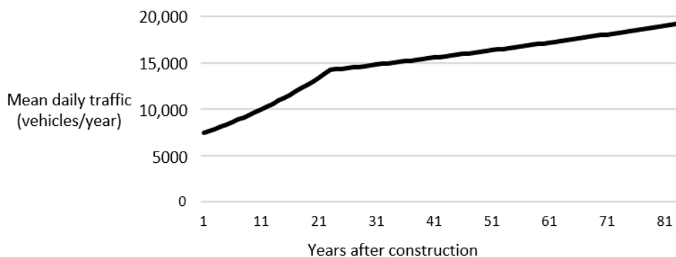
Figure A1. Estimated mean daily traffic on the bridge per year over the RSL (up to 80 years after construction).
