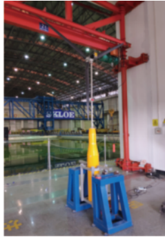
Fig. 12. COG adjustment of 6MW Spar type FOWT model system.
