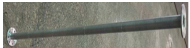
Fig. 6. Model tower with the length of 1.28 m.
