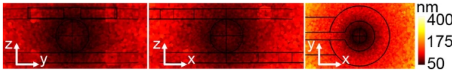
Figure D5. Mesh element size of the FEM-3D model for a superconducting sphere in an AHC-trap, with the maximum element size on the particle surface set to 50 nm. Parameters as in figure 3.
