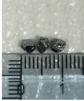
Figure 3.1: Single crystals Ba_8(Al_xGa_{1-x})_{16}Ge_{30} with well-defined facets grown by the flux method.
