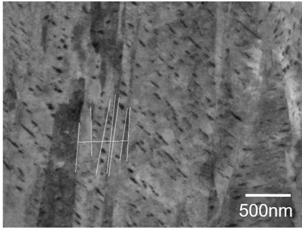
Fig. 1—Illustration of plate thickness measurements on SEM ECCI images.
