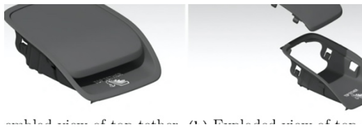
Fig. 2. Components-level views of the top tether.
