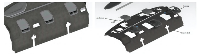
Fig. 3. System level views of the top tether.
