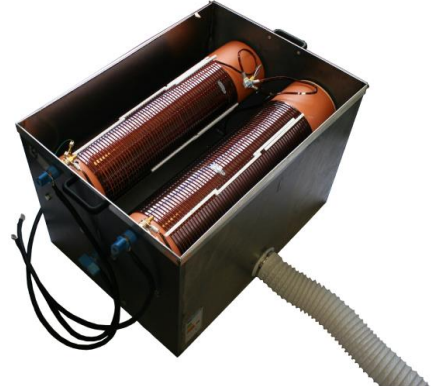
Fig. 10: Three-phase RL-load, air-core coil with forced air cooling.
