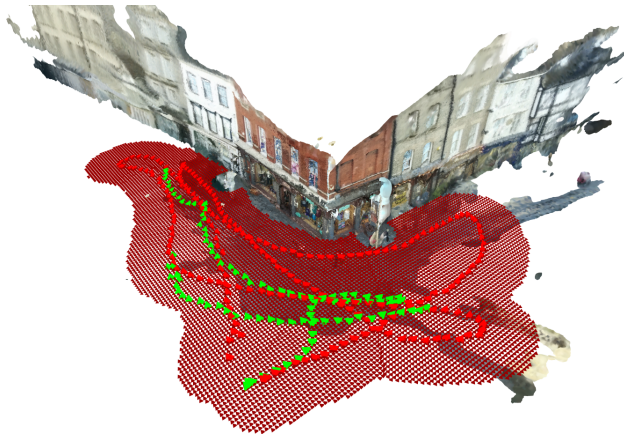
Figure 3. Visualization of synthetic generated poses for the rendered respectively translated images (dark red), poses of the captured training images (red) and poses of the captured test images (green).
