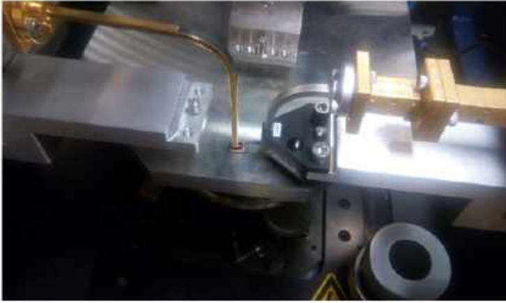
Figure 5.31: Measurement setup for the interconnect with the waveguide bend on the left and waveguide probe on the right (Paper D)
