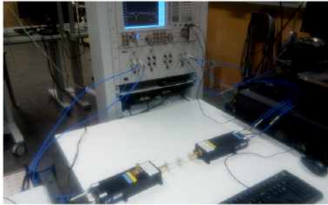
Figure 5.13: Measurement setup for TS transition (Paper C)
