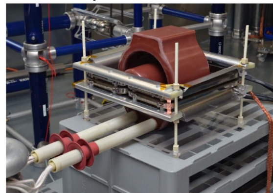
240 kVA, 0.6/0.9 kV, 10 kHz Grading et al. (ABB), 2017 [10] Claimed HV insulation to ground 50 kV DC PD free AC 50 Hz 35 kV
