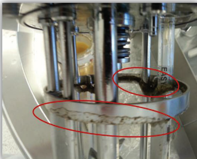
FIGURE 5.1 A black substance was observed after high respiratory activity was achieved under respiration-permissive conditions (Johanson et al., unpublished data).
