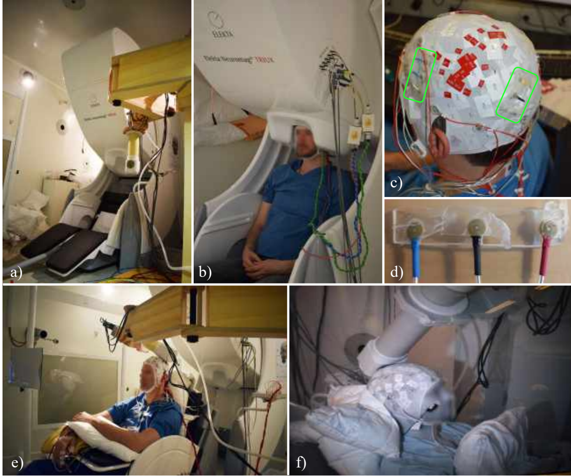
Figure 5.6: Photographs from the MEG measurements at NatMEG in Stockholm. a) The Elekta Neuromag TRIUX low- T_c SQUID-based full-head MEG system in the background and our 7-channel high- T_c SQUID-based system on the wooden fixture. b) Subject in the low- T_c SQUID system. c) EEG cap with EEG electrodes (with red cables), magnetic dipole-like coils for sensor localization highlighted in green, and red markings for cryostat positioning. d) Close-up photograph of the magnetic dipole-like coils. e) Subject prepared for a high- T_c SQUID recording. f) Subject during a high- T_c SQUID recording as seen through the MSR camera.
