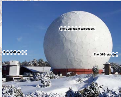
The collocated techniques of Very Long Baseline Interferometry (VLBI), the Global Positioning System (GPS) and Water Vapour Radiometry (WVR) at the Onsala Space Observatory on the west coast of Sweden.
