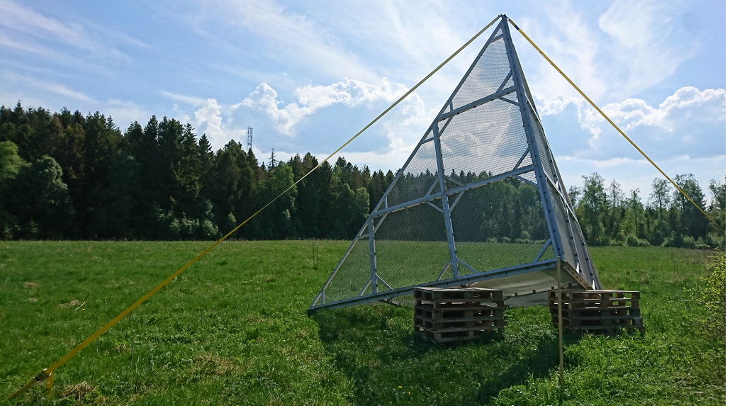
Figure 5.9. Photo of the trihedral corner reflector used for calibration (Trihedral corner 2 in Figure 5.1).
