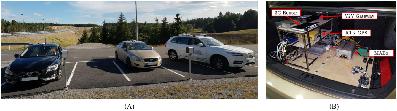
FIGURE 3 Photos of the experimental hardware platform. A, Shows the three vehicles used, B, shows the hardware installation in one of the vehicles. The 3G router was used to provide an IP link for the real-time kinematic corrections used by the GPS receiver [Colour figure can be viewed at wileyonlinelibrary.com ]
