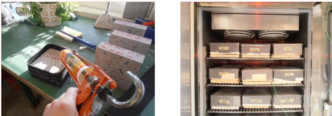
Figure 7. Preparation of salt-frost scaling tests. Left: Application of the rubber cloth and silicone sealant on the test specimens; Right: Salt-frost scaling test specimens placed in the climate chamber.
