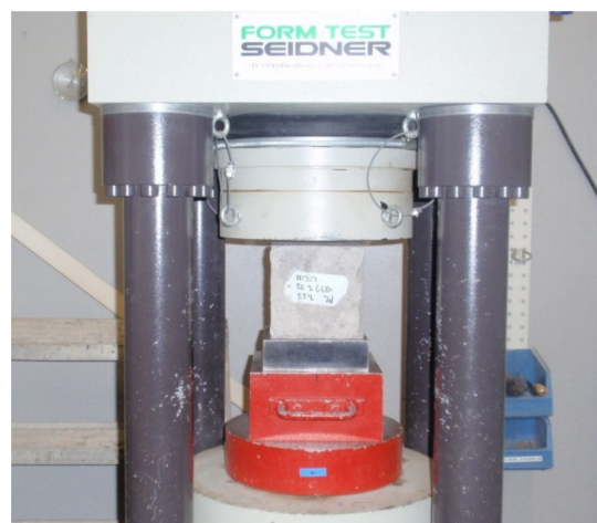
Figure 9. Compressive strength test set-up.
