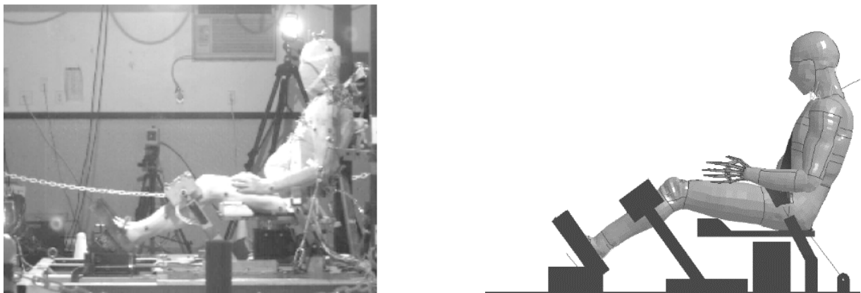
Fig. 4. Front sled test 40 km/h. Left : PMHS 1,358 (adopted from [25]). Right : corresponding FE simulation model.
