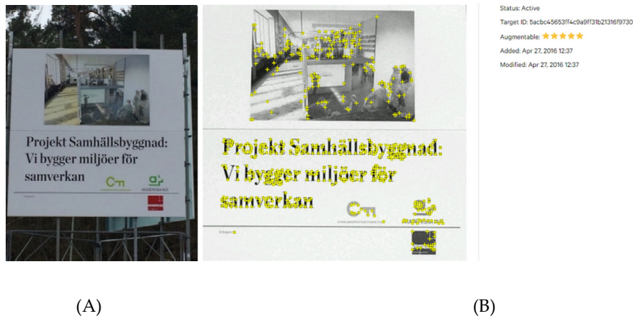
Figure 3. Display placard (A) used for P5, (B) shows the Vuforia's rating for recognizability of the placard as a tracker based on the patterns in the display.
