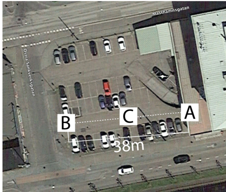
Figure 5. Placement of markers on-site for P7, markers were (A) 1.8 m × 1.8 m (A), and (B) and (C) 0.9 m × 0.9 m in size.
