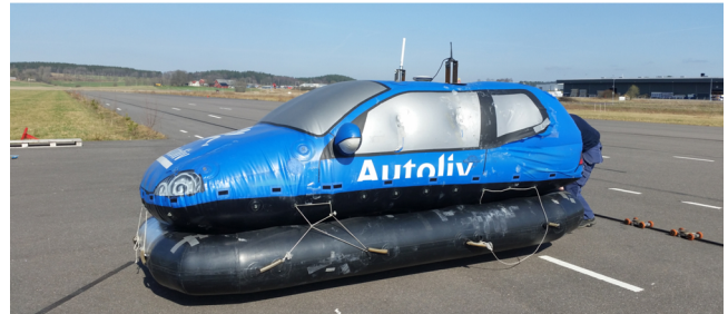
Fig. 1. The test-track experiment at Vårgårda airfield: The ego vehicle is approaching the cyclist dummy, mounted on a high-speed platform (panel a). Panel b shows the balloon vehicle used as an oncoming vehicle. A video of the trial is available: https://youtu.be/AixQ189hMi4 .
