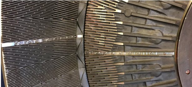
Figure 3: Two sensor arrays for temperature measurements mounted on the stator side (FZ-to the right and CD-to the left) in a CD76-TMP refiner. The chips are introduced in the central part of FZ.
