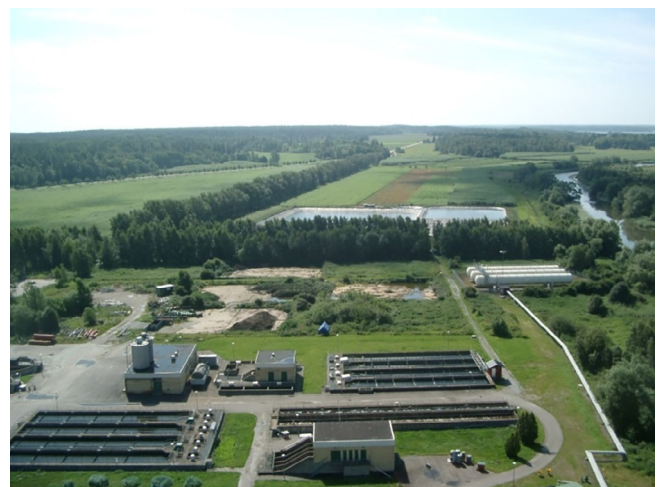
FIGURE 2 Overview of the system near Enköping, Sweden, where willow fields, irrigated by a municipal wastewater plant, supply a combined, heat and power plant (from where the photo is taken) with biomass (Photo: Pär Aronsson, SLU)
