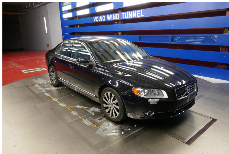
Figure 9. The reference vehicle mounted in the test section at zero yaw.
