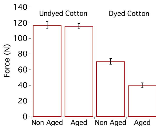
Figure 1. Maximum force at break of model cotton samples, undyed and dyed with iron-tannate dyes before [67] and after 10 years of natural ageing. From 5 to 10 tensile measurements per sample were carried out.
