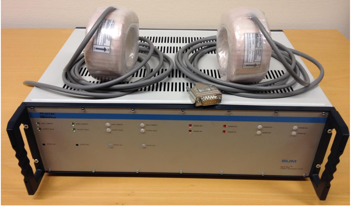
Figure 8: Photo of 500A/5V SUM (type 2ST20) system.
