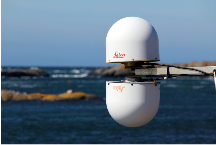
Figure 1.2: The two-antenna GTGU installation at the Onsala Space Observatory has a clear view of the sea surface. The upward antenna receives right-hand circularly polarized (RHCP) signals, and the downward antenna receives left-hand circularly polarized (LHCP) signals.
