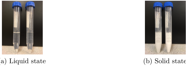
Figure 1.1: Phase change of two commercial PCMs (left sample holder: salt hydrate, right sample holder: paraffin)
